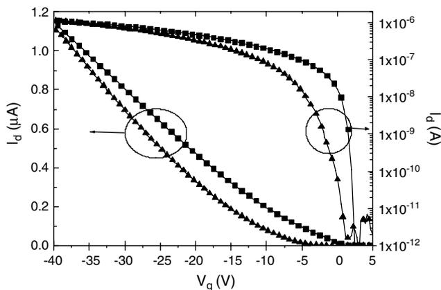
Fig. 1. Experimental transfer characteristics of BC (squares) and TC (triangles) pentacene TFTs, measured in vacuum at  $V_{\text{ds}} = -1 \text{ V}$  ( $L = 100 \mu\text{m}$ ,  $W = 200 \mu\text{m}$ ,  $d_{\text{ox}} = 150 \text{ nm}$ ).
