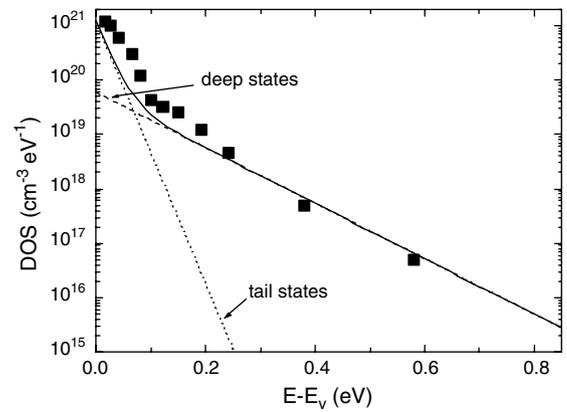
Fig. 6. Density of localized states calculated by the ‘temperature method’ (symbols). Solid line represents the approximated DOS used for the numerical simulations.
