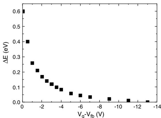
Fig. 5. Plot of the activation energy,  $\Delta E$ , derived from the Arrhenius plot of  $dG'/dV_g$ , vs  $V_g - V_{fb}$ . The flat band voltage,  $V_{fb} = 0.1$  was calculated by the method reported in Ref. [12].
