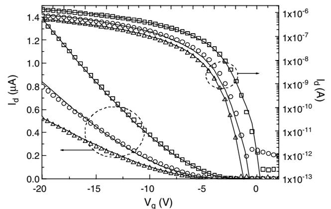
Fig. 3. Simulated (lines) and experimental (symbols) transfer characteristics (measured in vacuum at  $V_{\text{ds}} = -1 \text{ V}$ ), of as-fabricated TC pentacene TFTs for three different temperatures: 300 K (squares), 240 K (circles), 205 K (triangles) ( $L = 100 \mu\text{m}$ ,  $W = 200 \mu\text{m}$ ,  $d_{\text{ox}} = 60 \text{ nm}$ ).
