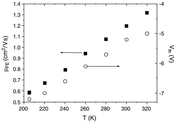
Fig. 4. Field effect mobility,  $\mu_{FE}$ , and threshold voltage,  $V_{th}$ , vs temperature of TC pentacene TFT.
