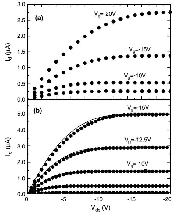
Fig. 2. Experimental (symbols) output characteristics of BC (a) and TC (b) pentacene TFTs, measured at  $T = 300 \text{ K}$  and different gate voltages ( $L = 100 \mu\text{m}$ ,  $W = 200 \mu\text{m}$ ,  $d_{\text{ox}} = 60 \text{ nm}$ ). Also shown are the simulated output characteristics of TC pentacene TFT (b, solid lines).
