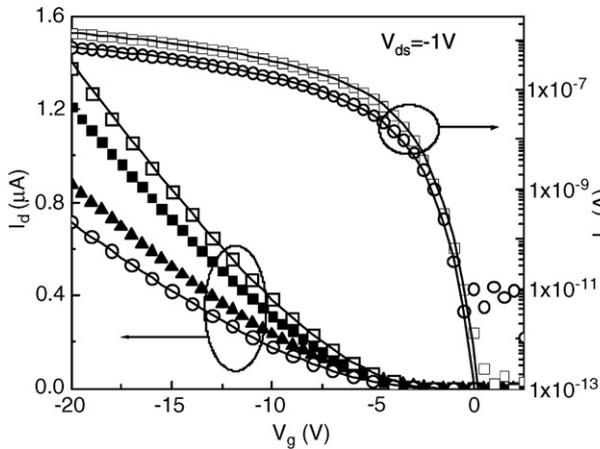
Fig. 5. Experimental transfer characteristics (symbols), measured in vacuum at  $V_{ds} = -1$  V, for as-fabricated devices (open squares) and after 2 (closed squares), 15 (closed triangles) and 40 (open circles) days. ( $L = 100$   $\mu\text{m}$ ,  $W = 200$   $\mu\text{m}$ ). Solid lines are the calculated transfer characteristics fitting the as-fabricated and 40-days conditions.
