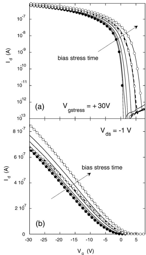
Fig. 2. Experimental transfer characteristics measured at different bias stress times ( $0-10^4$  s) (solid lines) and after 48 h (dashed line). Bias stress condition  $V_{g\text{stress}} = +30$  V;  $V_{ds} = -1$  V. Transfer characteristics, calculated by the trap states model, are also shown, corresponding to unstressed (closed circles), after bias stress (open circles) and recovered device (open squares).
