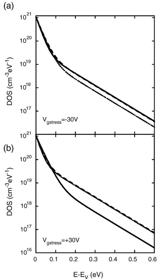
Fig. 4. Density of localized states calculated by fitting transfer characteristics of Figs. 1 (a) and 2 (b), corresponding to negative and positive bias stress, respectively. Solid lines: unstressed devices; dashed lines: after bias stress devices; dot lines: recovered devices.
