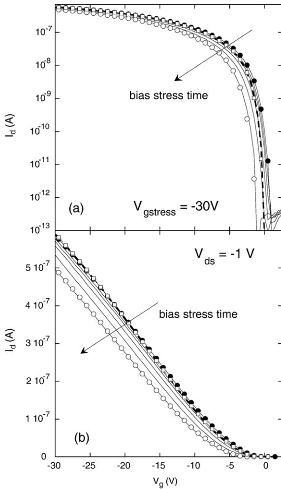
Fig. 1. Experimental transfer characteristics measured at different bias stress times ( $0-10^4$  s) (solid lines) and after 48 h (dashed line). Bias stress condition  $V_{g\text{stress}} = -30$  V;  $V_{ds} = -1$  V. Transfer characteristics, calculated by the trap states model, are also shown, corresponding to unstressed (closed circles), after bias stress (open circles) and recovered device (open squares).
