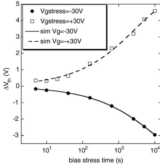
Fig. 3. Threshold voltage variation ( $\Delta V_{th} = V_{th}(t) - V_{th}(0)$ ) for pentacene OTFTs during positive (squares) and negative bias stress. Stretched exponential functions (lines), fitting experimental data, are also shown.
