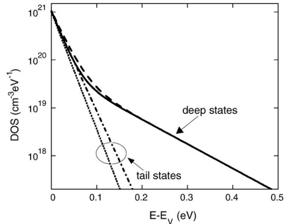
Fig. 7. Density of localized states calculated by fitting transfer characteristics of Fig. 5, corresponding to as-fabricated device (solid line) and the device aged for 40 days (dashed line). Tail states components for as-fabricated (dot) and aged device (dashed-dot) are also shown.
