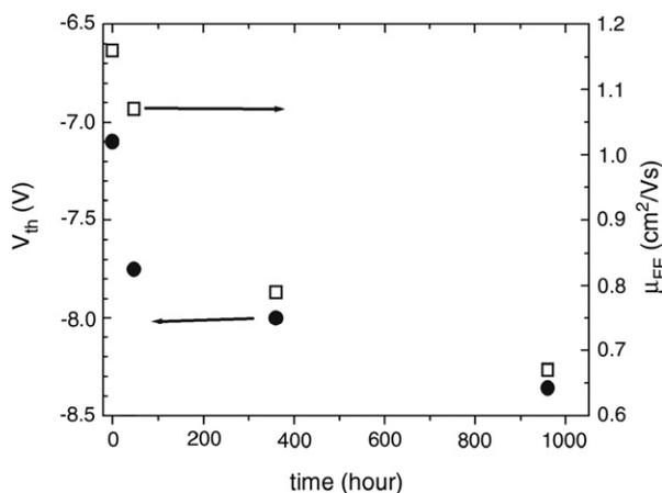
Fig. 6. Threshold voltage and field effect mobility variations during 40 days for a pentacene OTFTs in air.  $V_{th}$  and  $\mu_{FE}$  are calculated from the transfer characteristics shown in Fig. 5.
