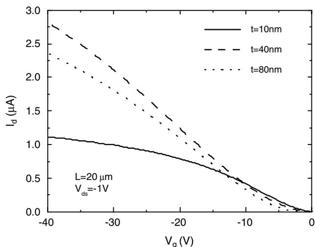
Fig. 2. Transfer characteristics of pentacene BC-TFTs with different pentacene thickness and  $L = 20$   $\mu\text{m}$ .
