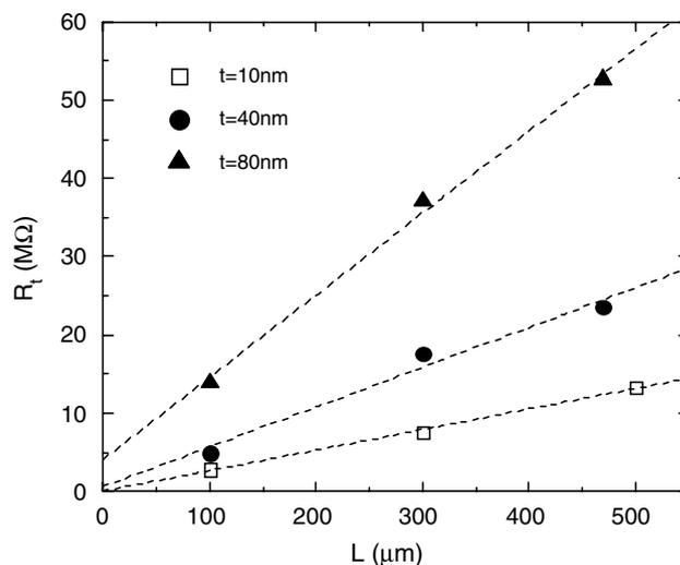
Fig. 8. Total channel resistance vs channel length for pentacene TC-TFTs with different active layer thickness.
