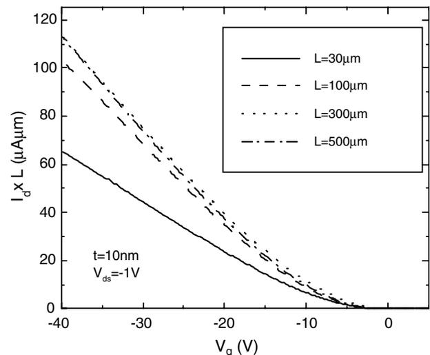
Fig. 6. Transfer characteristics, normalized to channel length, for pentacene TC-TFTs with  $10$  nm pentacene thickness.
