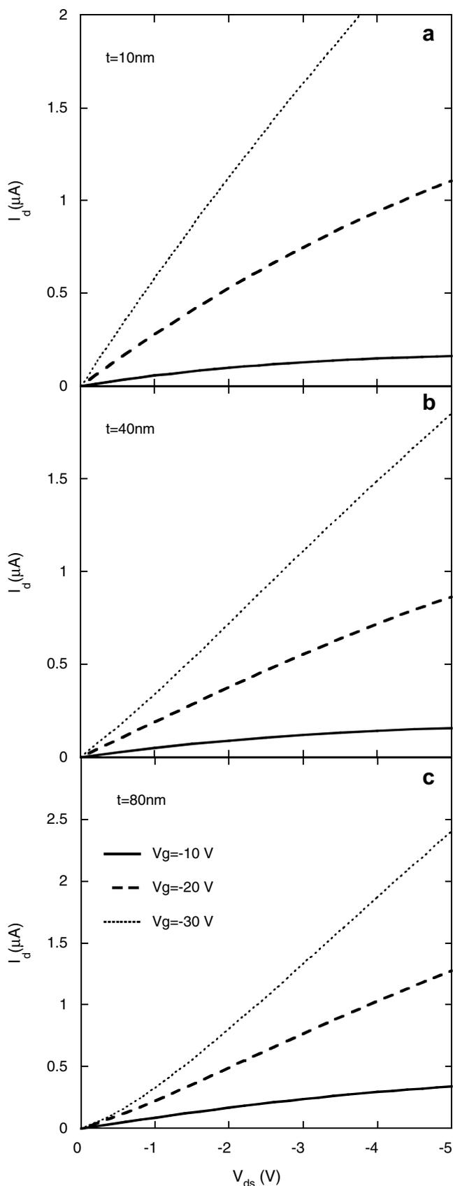
Fig. 7. Output characteristics of pentacene TC-TFTs with  $L = 100 \mu\text{m}$  and different pentacene thickness, measured at  $V_g = -10, -20$  and  $-30 \text{ V}$ .
