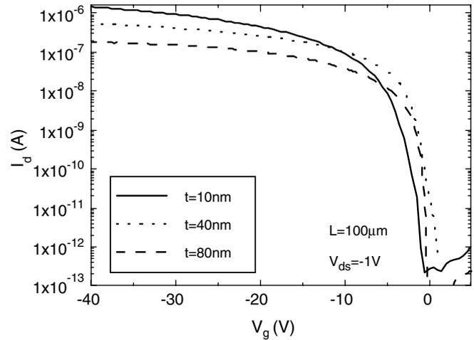
Fig. 5. Transfer characteristics of pentacene TC-TFTs with different pentacene thickness and  $L = 100$   $\mu\text{m}$ .
