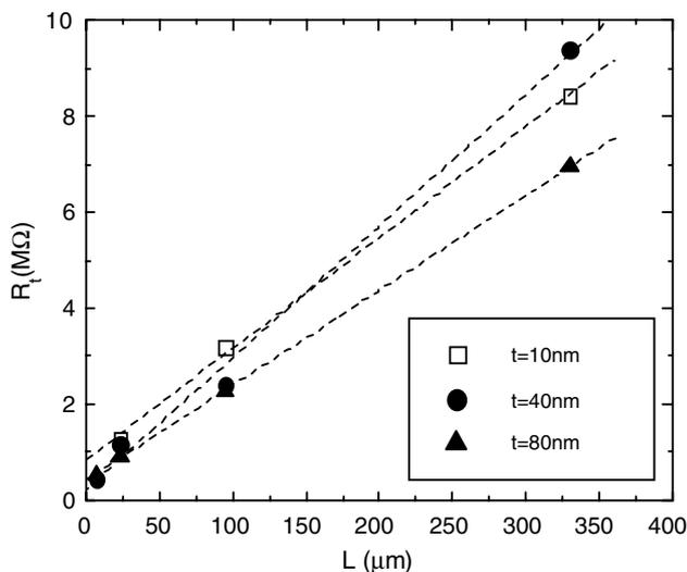
Fig. 4. Total channel resistance vs channel length for pentacene BC-TFTs with different active layer thickness, calculated at  $V_g = -20$  V and  $V_{ds} = -1$  V.
