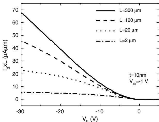
Fig. 1. Low voltage ( $V_{ds} = -1$  V) transfer characteristics, normalized to channel length, for pentacene BC-TFTs with 10 nm of pentacene thickness.
