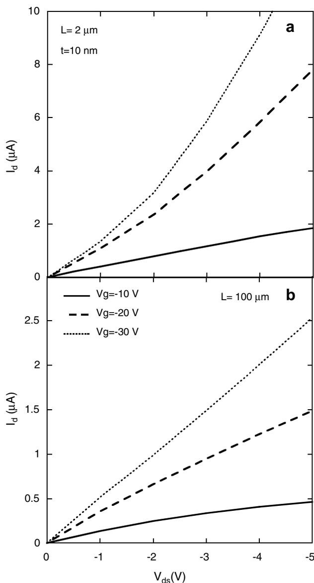
Fig. 3. Output characteristics of pentacene BC-TFTs with  $t = 10$  nm and two different channel lengths,  $L = 2$   $\mu\text{m}$  (a) and  $L = 100$   $\mu\text{m}$  (b), measured at  $V_g = -10, -20$  and  $-30$  V.
