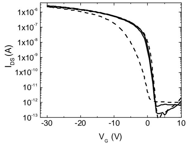
**Fig. 3:** Experimental up-down transfer characteristic ( $V_{DS} = -1$  V) of annealed device, measured in vacuum (solid line) and in air (dashed line).
