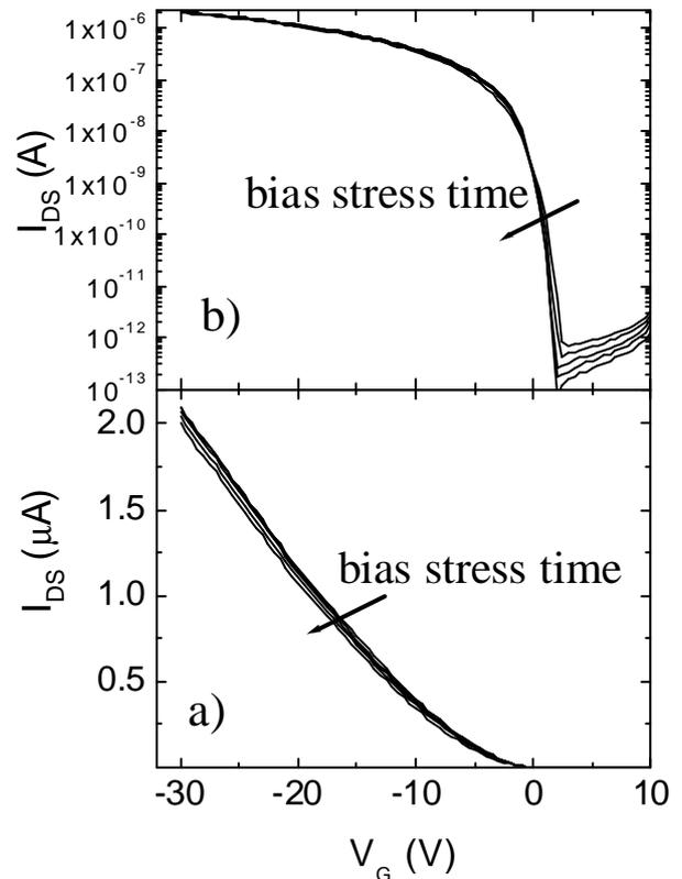
**Fig. 4:** Experimental transfer characteristics measured in vacuum on pentacene patterned and annealed device at different bias stress time (0- $10^4$  s). Bias stress condition  $V_{Gstress} = -30$  V,  $V_{DS} = -1$  V.
