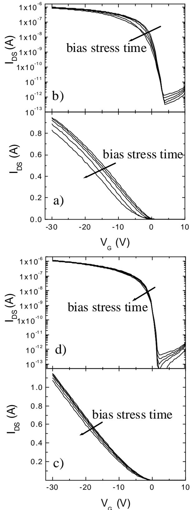
**Fig. 6:** Experimental vacuum transfer characteristics measured on pentacene patterned aged and not annealed device (a-b), and on aged but annealed device (c-d) at different bias stress time ( $0-10^4$ s). Bias stress condition  $V_{Gstress} = -30V$ ,  $V_{DS} = -1V$ .
