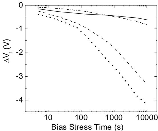
**Fig. 5**  $V_T$  shift for conventional un-passivated (dotted line), and passivated and annealed TFTs (solid line). Also shown is the  $V_T$  shift for passivated and aged TFTs before (dashed) and after (dot-dashed) thermal annealing.
