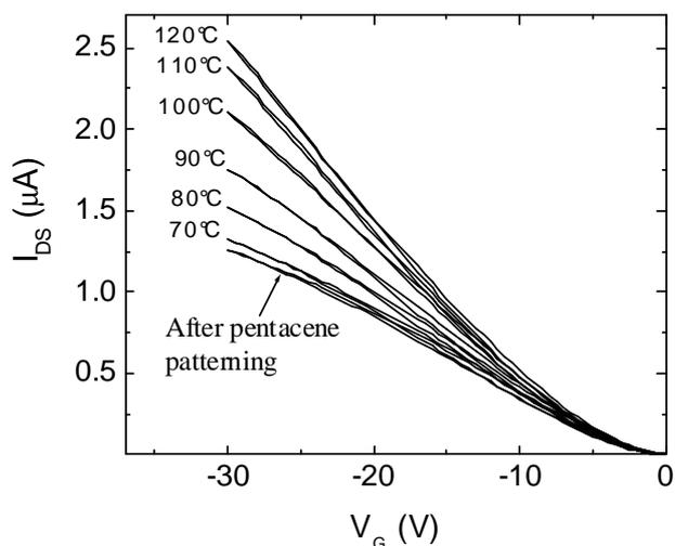
Fig. 2: Experimental up-down transfer characteristics, measured in vacuum, after the pentacene patterning for different annealing temperatures.
