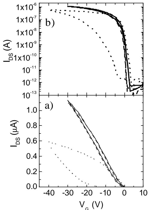
Fig. 1: Experimental transfer characteristics, measured in vacuum ramping up-down the gate bias, before parylene deposition (solid line), after pentacene patterning (dashed line) and after pentacene patterning, measured in air (dotted line).
