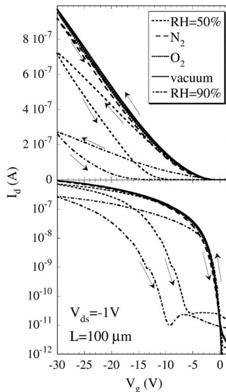
Fig. 3. Transfer characteristics of pentacene TFTs measured under different environmental conditions (shown in the label).
