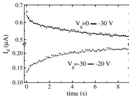
Fig. 4. Time dependence of the drain current of a pentacene TFT, measured in air, after changing gate voltage from 0 V to -30 V (squares) and after changing  $V_g$  from -30 V to -20 V (triangles).  $I_d$ -curves are fitted by two-exponential decay functions (solid lines).
