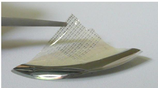
Fig. 2. Photograph of polyimide substrate with pentacene TFTs after released from the rigid carrier.
