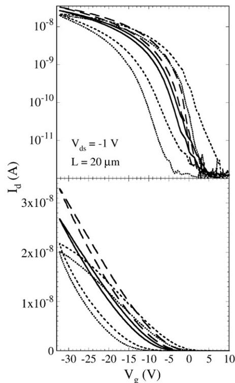
**Fig. 6.** Transfer characteristics of pentacene TFTs on plastic substrate measured in vacuum and air for devices without acryl layer (solid and short dashed lines) and with acryl encapsulation (long dashed and dot lines).
