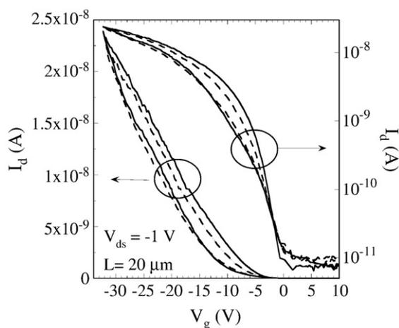
Fig. 7. Transfer characteristics of pentacene TFTs on plastic substrate, with Al encapsulation layer, measured in vacuum (solid line) and in air (dashed line).
