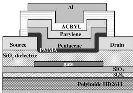
Fig. 1. Cross sectional view of a bottom contact pentacene OTFT fabricated on polyimide substrate.
