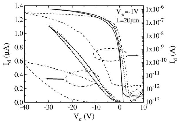
**Fig. 5.** Transfer characteristics of pentacene TFTs measured at  $V_{ds} = -1$  V, sweeping gate voltage from positive to negative values and back: before parylene deposition (solid line), after pentacene patterning (dot line), both measured in vacuum, and after pentacene patterning, measured in air (dashed line).
